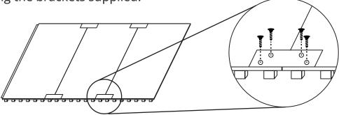
If you purchased multiple sprung kits to connect together, you only need to install the brackets between the panels along the outer edges.
